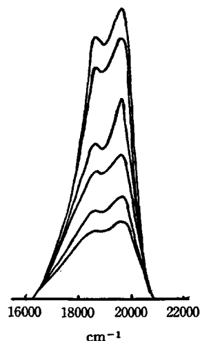
Fig. 6. Phosphorescence spectra of p -nitroaniline. the uppermost curve: added 0 M cinnamic acid the second curve: added 0.01 M cinnamic acid the third curve: added 0.05 M cinnamic acid the fourth curve: added 0.1 M cinnamic acid the fifth curve: added 0.15 M cinnamic acid the lowest curve: added 0.2 M cinnamic acid
